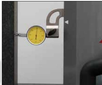
Squariness mechanically adjusted on all instruments
