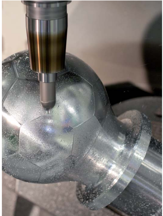
Five-axis manufacturing of the Telstar World Championship ball of 1970 and 1974
