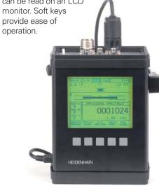
The **PWT** is a simple adjusting aid for HEIDENHAIN incremental encoders. In a small LCD window the signals are shown as bar charts with reference to their tolerance limits.
