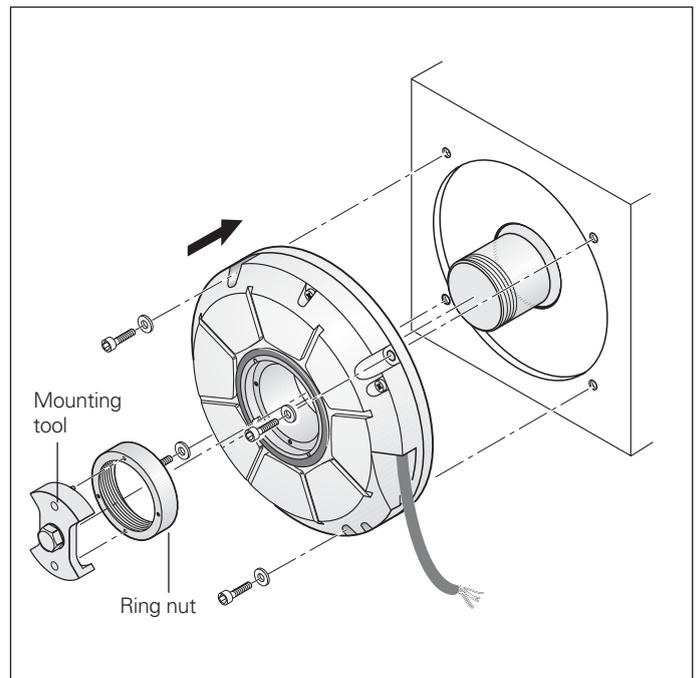
Mounting an angle encoder with hollow through shaft
