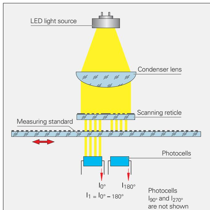
**Interferential scanning principle**
