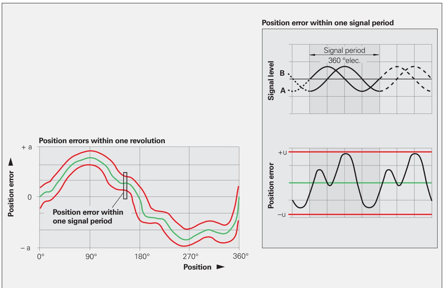
For its angle encoders with integral bearings, HEIDENHAIN prepares individual calibration charts and ships them with the encoder.
