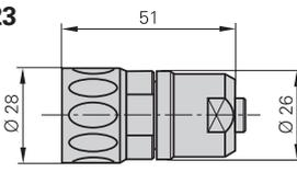
Insulated **coupling**: Connecting element with external thread; available with male or female contacts.
