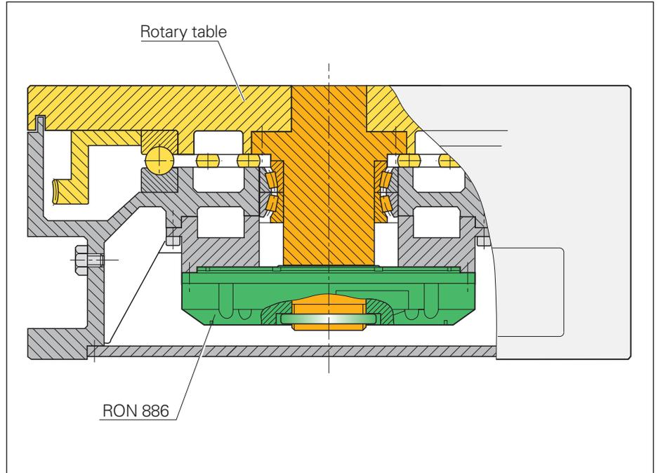
The **RON 886** angle encoder mounted onto the rotary table of a machine tool
