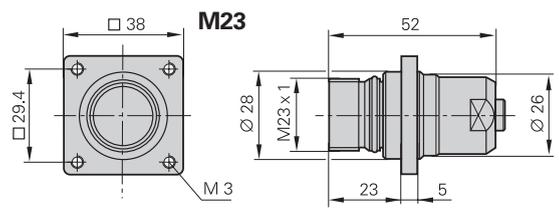
**Flange socket**: Permanently mounted on the encoder or a housing, with external thread (like the coupling), and available with male or female contacts.
