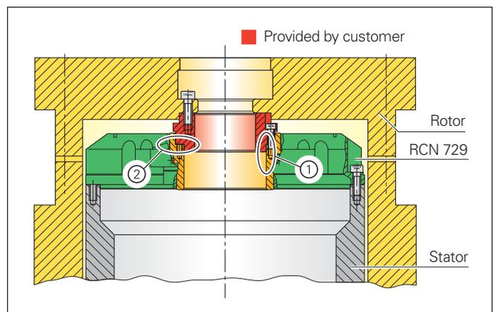
Front-end shaft coupling with **RCN 729**
